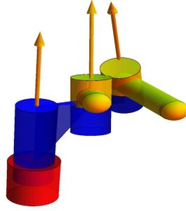
**Fig. 5** The two-fingered design for the first two finger tasks in Figure 2**Table 4** Joint axes for the 1 - (1, 1) hand designed for the first two fingers of the task in Figure 2.
