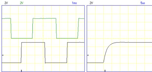
Figure 5: Oscilloscope trace of two channel encoder
